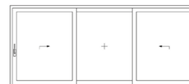
three-part element with two lift/sliding sashes and fixed glazing
