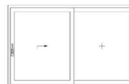
two-part element with lift/sliding sash and fixed glazing
